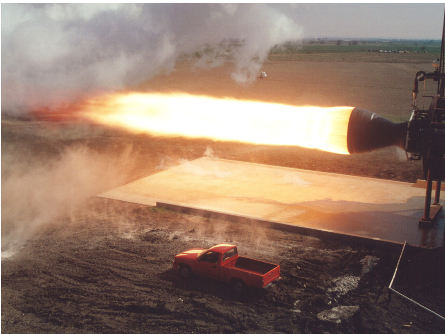
One of Beal Aerospace's engines undergoing a static test fire
